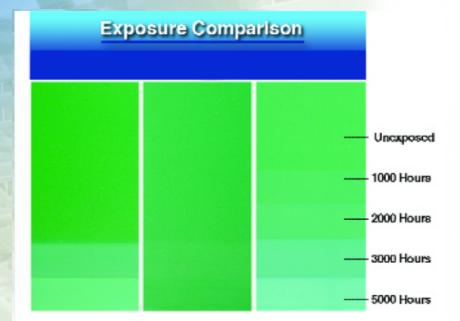
IR Heat Reflective coatings undergo extensive testing for fade resistance. Every 1000 hours of testing is equivalent to approximately one and a half years of exposure 5000 hours is equivalent to 8-10 years.
