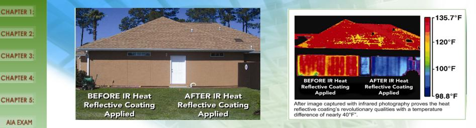
Infrared photography proves that IR heat reflective coatings provide greater heat reflectivity than traditional paints. In fact, IR heat reflective coatings can reduce a wall's surface temperature by nearly 40 degrees when compared to traditional paints in the same color.
