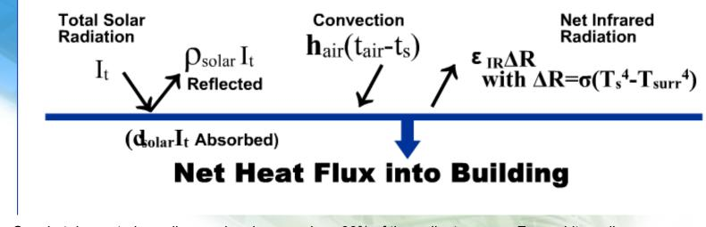
On a hot day, exterior walls can absorb as much as 90% of the radiant energy. Even white walls can absorb significant solar radiation. The wall's absorption of radiant energy makes the inside of the structure hotter and creates greater demand on HVAC systems, thus contributing to carbon emissions.
